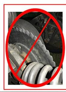
The picture to the left is showing the blade installed the incorrect way. The bevel should be outwards towards the depth wheel.
